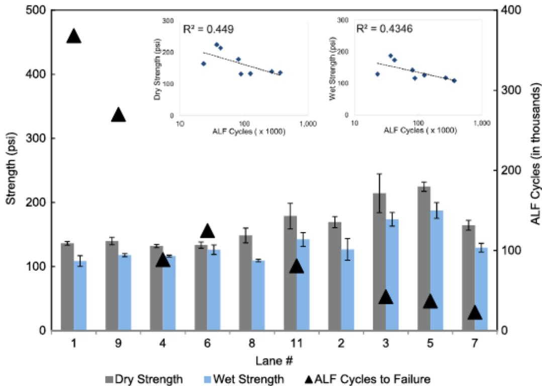
Figure 2. Correlation of IDT Strength (Dry and Wet) to ALF Cycles to Failure
