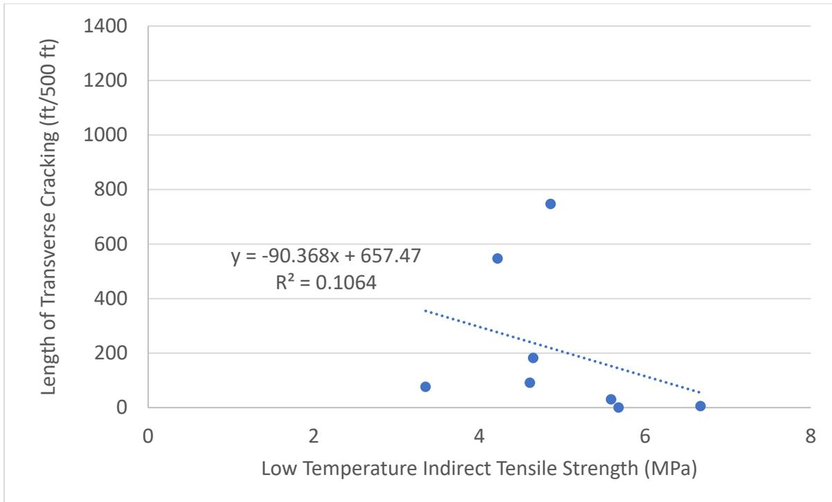
Figure 3. Correlation of IDT Strength (Low Temperature) to Length of Transverse Cracks
