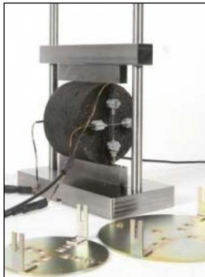
Figure 1. Indirect Tensile (IDT) Test Jig by Controls Group
